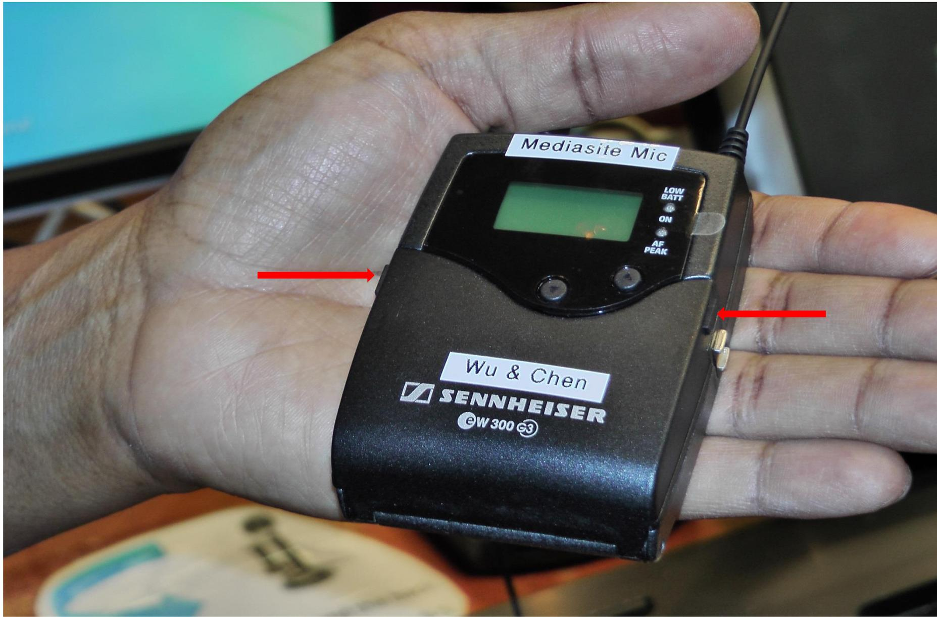
To access the power button, you will need to squeeze the two door release latches located on the sides.
